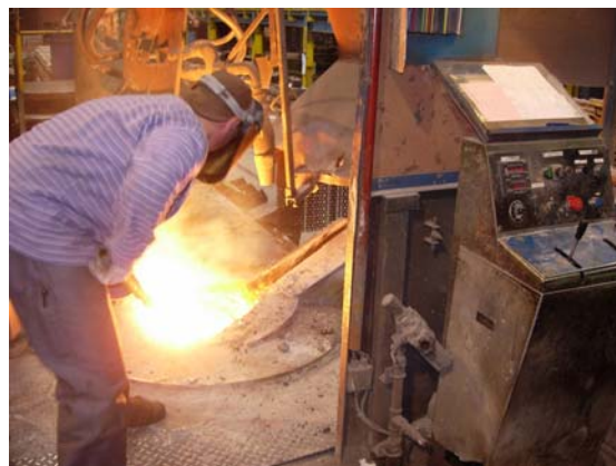
Operator working at open metal induction heater
