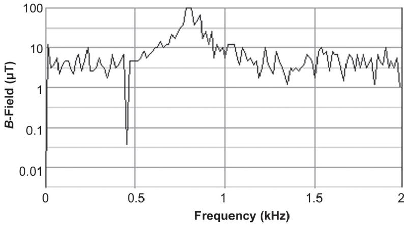
**Figure 5. Spectral analysis of induction heater No. 4.** Notes. Wide band at 70 cm from heater: 303  $\mu\text{T}$ ,  $B$ -field—magnetic flux density.
