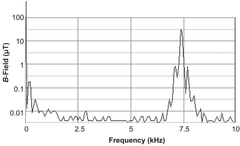
**Figure 4. Spectral analysis of induction heater No. 3.** Notes. Wide band: 107  $\mu\text{T}$ ,  $B$ -field—magnetic flux density.
