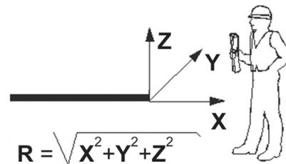
Figure 2. B-field polarization and resultant ( $R$ ) calculation.
