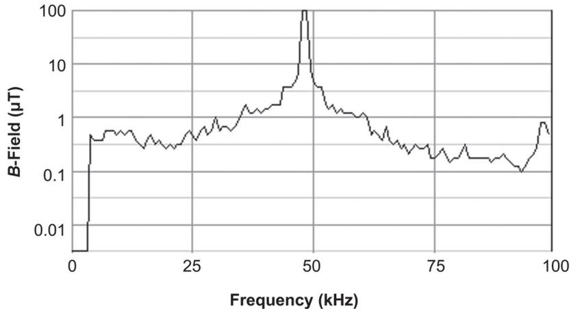
**Figure 8. Spectral analysis of induction heater No. 7.** Notes. Wide band at 4 m from heater: 116  $\mu\text{T}$ ,  $B$ -field—magnetic flux density.
