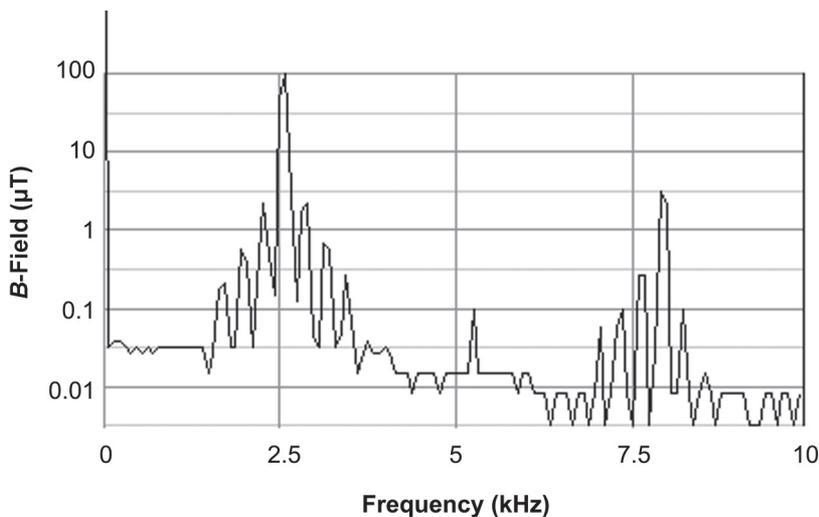
**Figure 3. Spectral analysis of induction heater No. 2.** Notes. Wide band: 107  $\mu\text{T}$ ,  $B$ -field—magnetic flux density.
