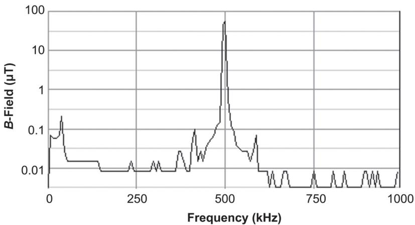
**Figure 6. Spectral analysis of induction heater No. 5.** Notes. Wide band at 60 cm from heater: 60  $\mu\text{T}$ ,  $B$ -field—magnetic flux density.
