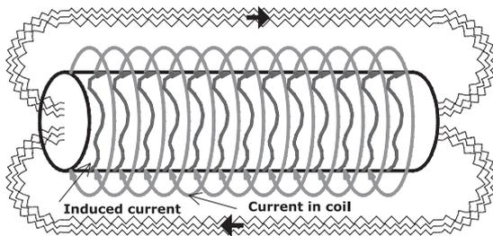
Figure 1. Principle of induction heating.
